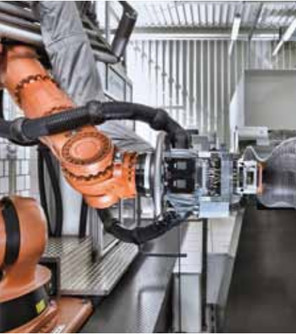
Fiber-Placement-Technologie am Fraunhofer IGCV
